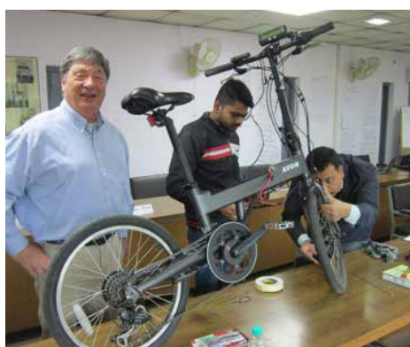
Installing Cycle Analyst data acquisition system on E-Bike for road test
