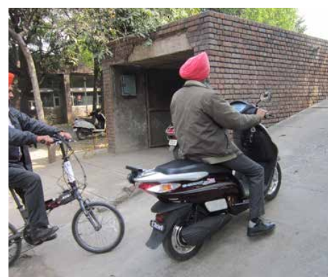
E-Scooter and E-Bike on 7-degree ramp test with data acquisition systems at RDCBSM
