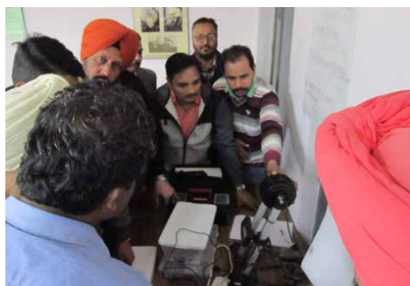
Hub motor test stand with Cycle Analyst display, data logger, C-M-T tester and 50-volt DC power supply
