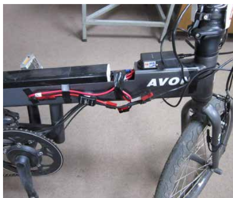
Data logger and current measurement shunt installed for road test
