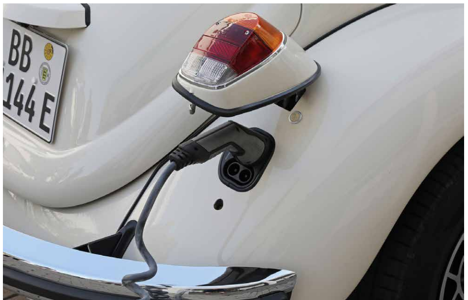
Note the CCS connector underneath the right taillight assembly!
