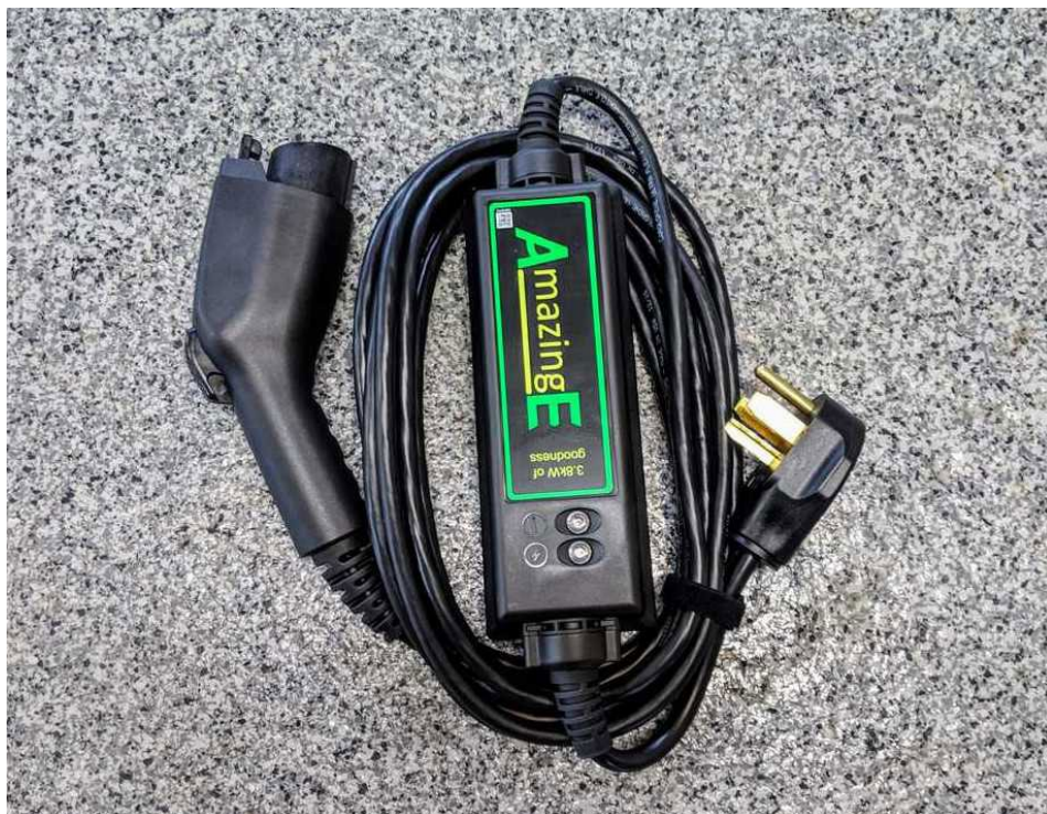
A lower-powered portable Level 2 charger. It's about the same size as a portable Level 1 unit, but can deliver much more power. *Notice a NEMA 14-30 240V plug is used.
