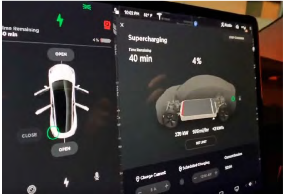
Version 3 Supercharger delivering 239 kW into Model 3 at nearly 1000 miles (of range gained) per hour! It really works!
