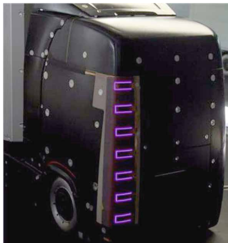
The KTH system uses plasma actuators mounted on the cab of the truck (Credit: KTH)
