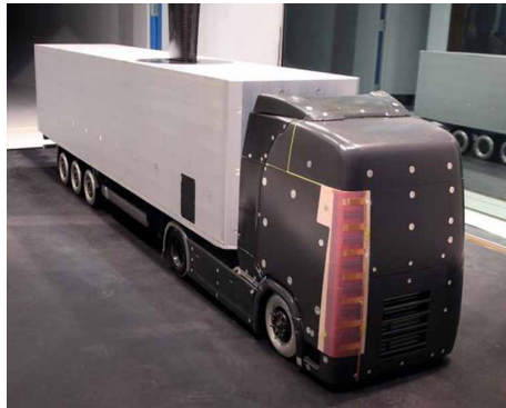
KTH is testing a system that uses electric winds to reduce fuel consumption in trucks (Credit: KTH)
