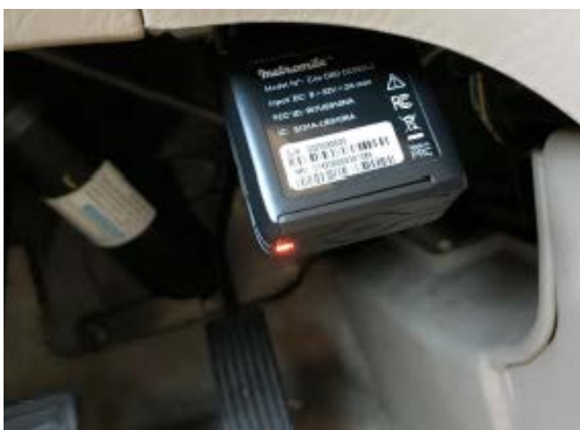
Figure 2 Installed and connected Dongle Just insert the dongle into the onboard diagnostic port (OBD_II) under the dash of your car. The dongle gets power from the port and "calls home" to report info about status of your car.
