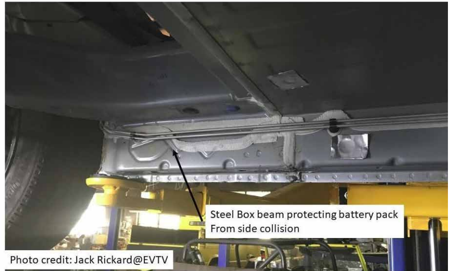
Steel Box Beam Protects Model 3 battery from side collision
