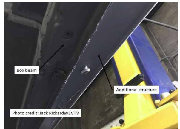
Bottom view of steel box beam and additional structure protecting battery from side collision
