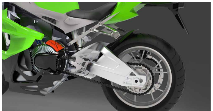
Lightweight and compact, the Magnax motor should be terrific in electric motorcycles where weight is paramount (Credit: Magnax)
