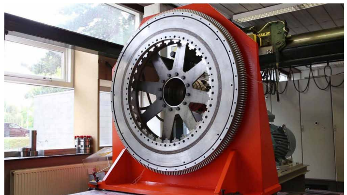
Large industrial-sized prototype on the test bench (Credit: Magnax)
