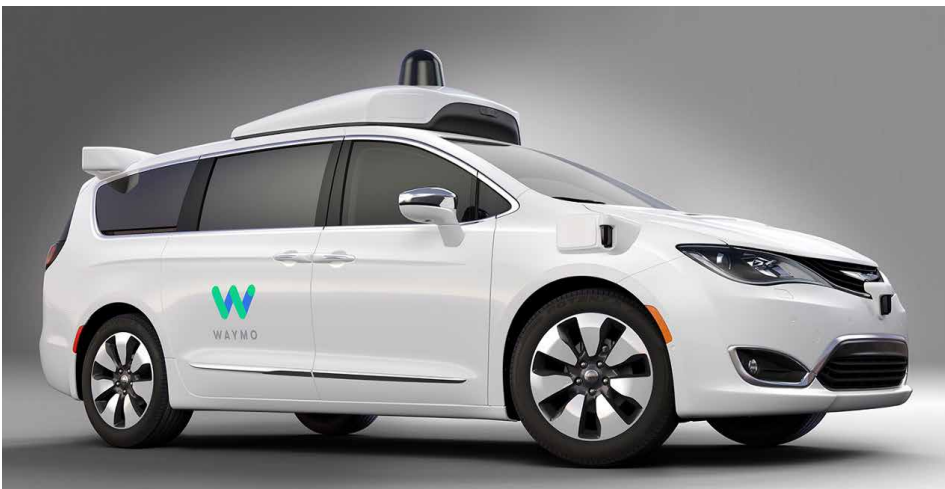
Waymo's AV minivan adds sensors and computing systems that increase weight, drag, and electrical power consumption. This model was used as an example of a 'large' sized AV system in the referenced study. Image source: Waymo
