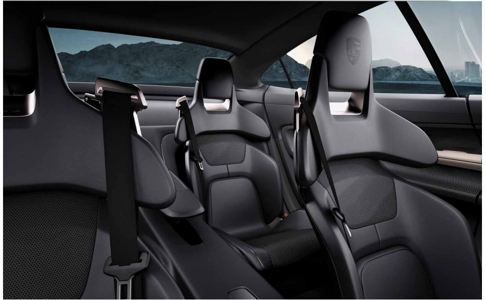
Four extremely lightweight individual seats provide excellent lateral support. (Photo: Porsche)
