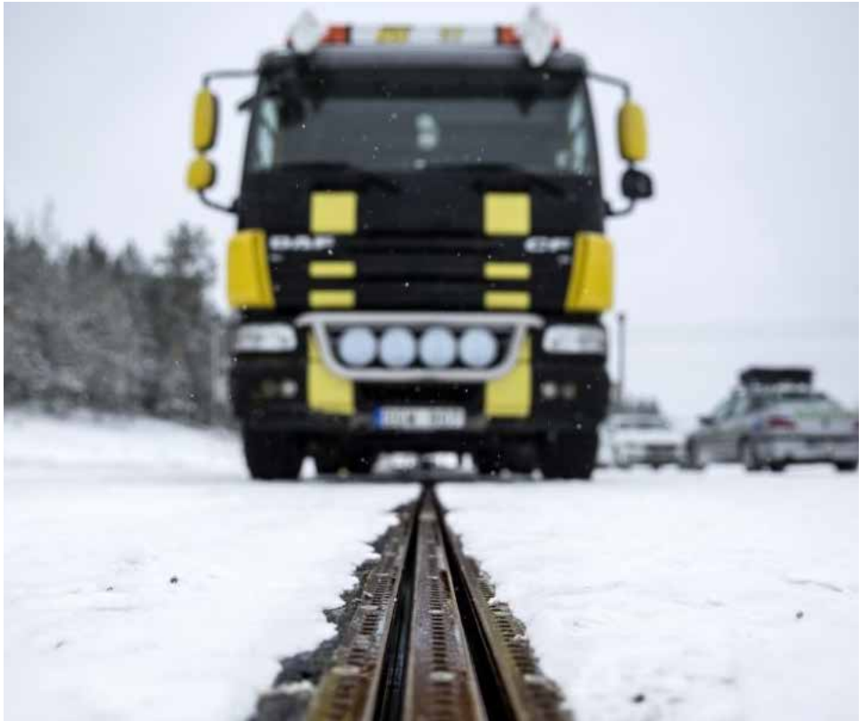
An electric truck drives down a snow-covered electrified road that charges the vehicle as it drives.
