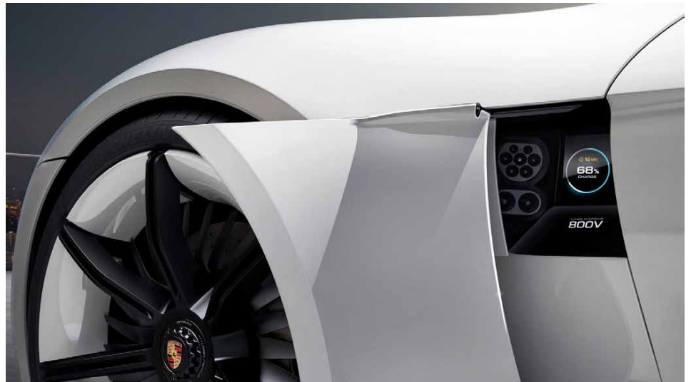
Part of the fender slides open to reveal the charging port. (Photo: Porsche)
