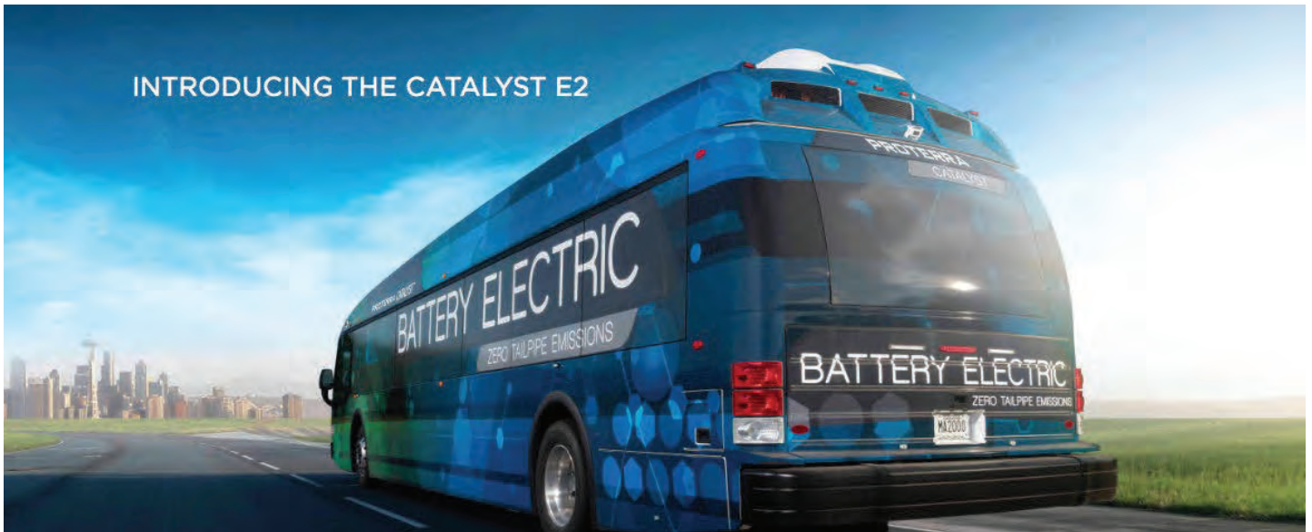
The Proterra Catalyst E2 has a claimed nominal range of 194 to 350 mi. (312 to 563 km) (Photo: Proterra)
