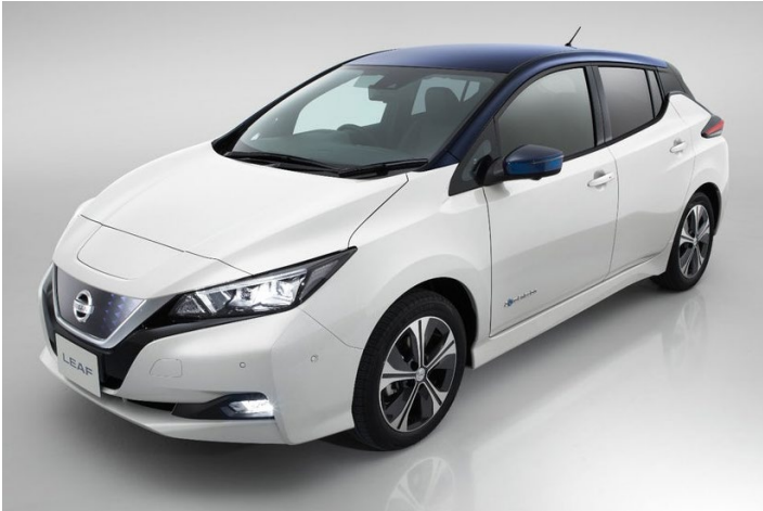
The new Leaf was inspired by the IDS Concept It has a drag coefficient of just 0.28
