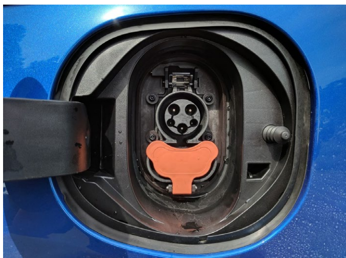
The Bolt's charge port isn't illuminated
