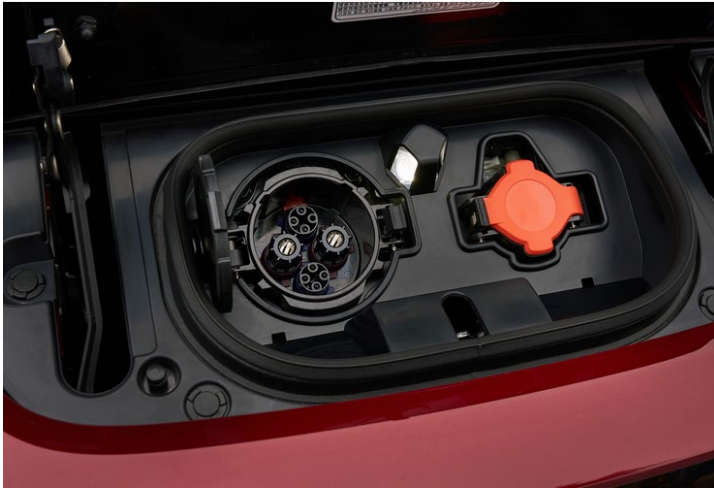
CHAdeMO standard for the US model based on the press pictures. (Photo Electrek)
