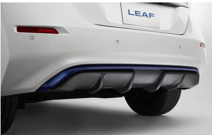
The latest Leaf has a 40 kWh battery pack and has 110 kW of power, as well as 320 Nm of torque. The diffuser on the helps contribute to a 0.28 Cd
