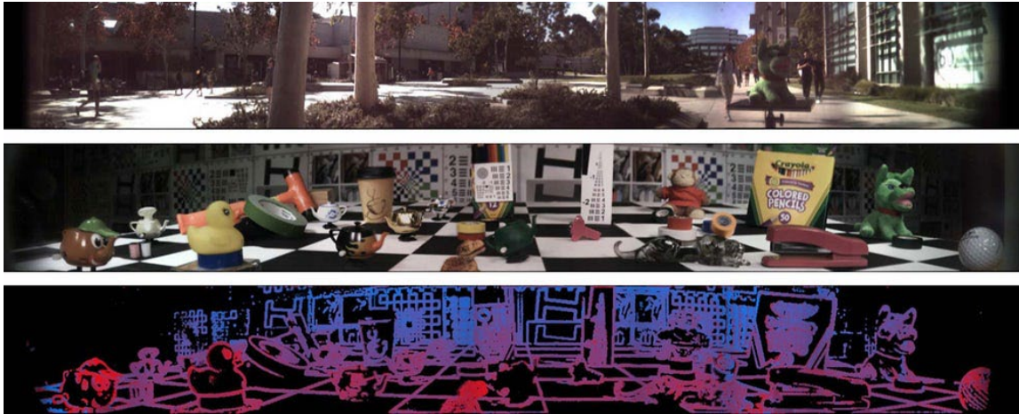
Two 138-degree light field panoramas (top and center) and a depth estimate of the second panorama (bottom)(Credit: Stanford Computational Imaging Lab/ Photonic Systems Integration Laboratory at UC San Diego)
