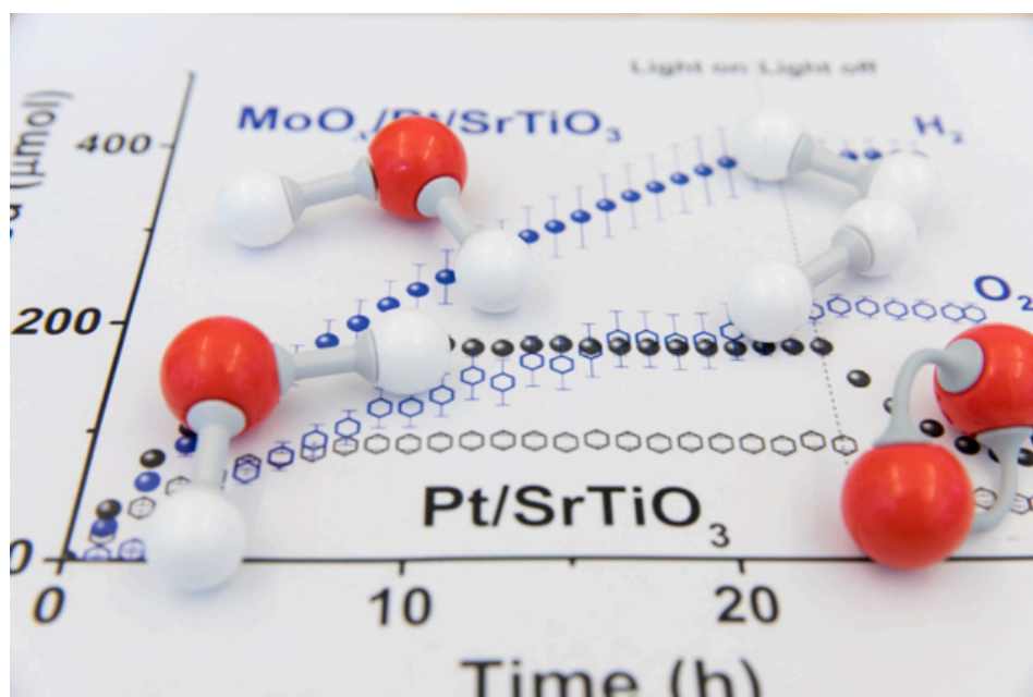
The graph shows hydrogen production over time, rising then leveling off with the non-coated catalyst, while the volume continually grows with the coated one. Photo from Andy Freeberg / SLAC National Accelerator Laboratory)
